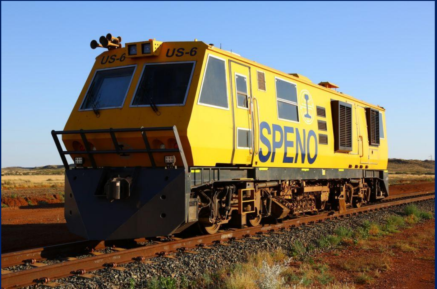
Speno ultra sonic rail flaw detector vehicle US-6 at Archers Siding May 13th. Photo Toad Montgomery
