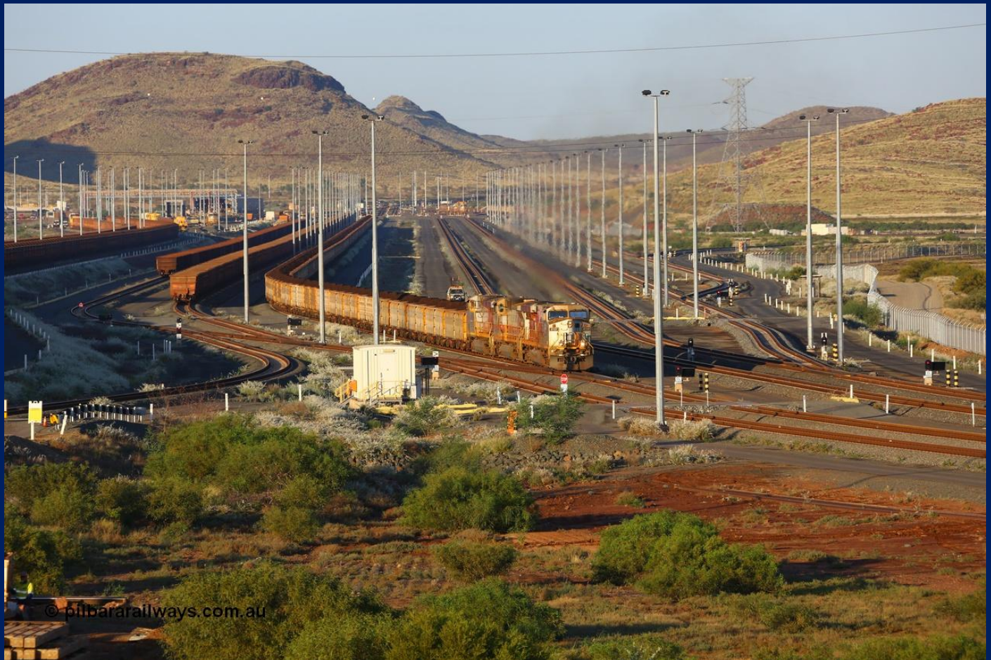
Cape Lambert South Yard with train of 2xES44DCi and C44-9W departing for port car dumpers May 10th.
