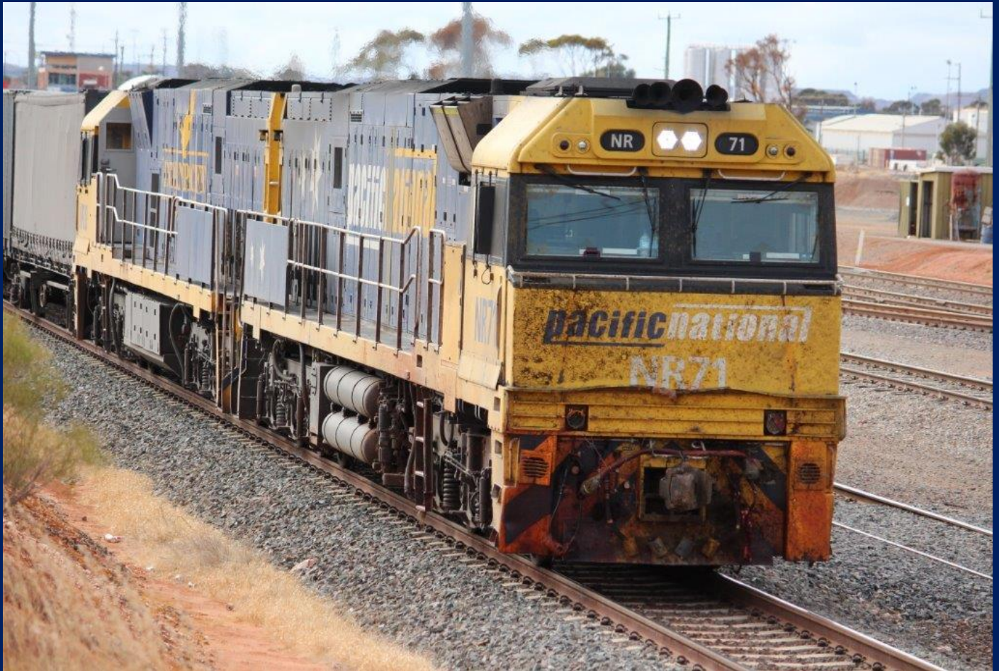
NR71 showing damage sustained when hit a cow on ARTC line on 6SP5 with NR26 West Kalgoorlie 25/6.
