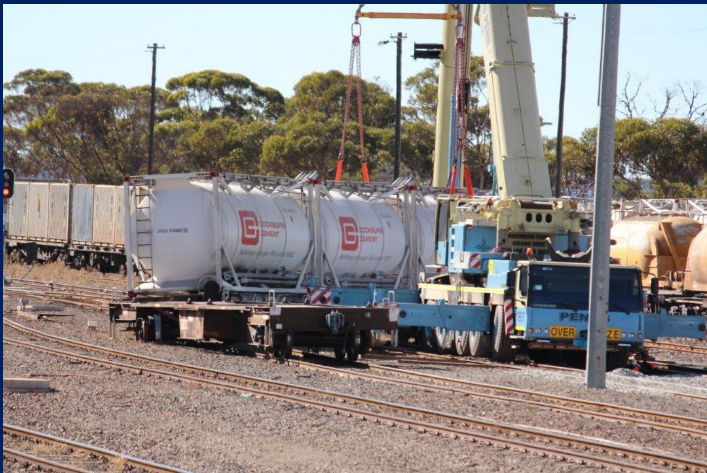
Transferring loading and re-railing wagons in West Kalgoorlie Yard 10/6.
