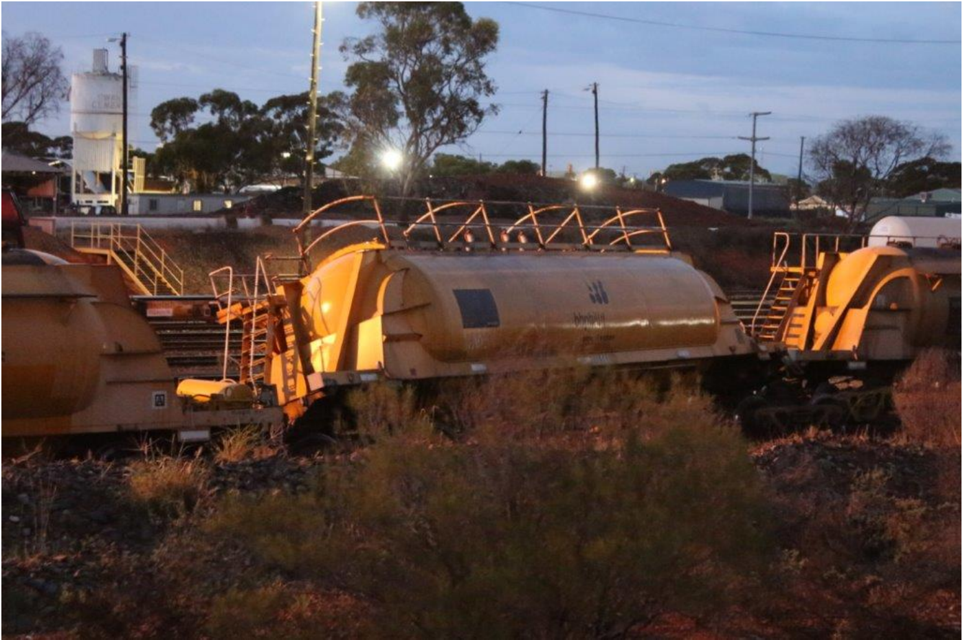
In the early hours of 16 th March, two empty WN nickel wagons on 2479 to Leonora split the points and derailed while departing West Kalgoorlie yard. Rerailing was completed that afternoon. Both photos: Peter Donaghy
