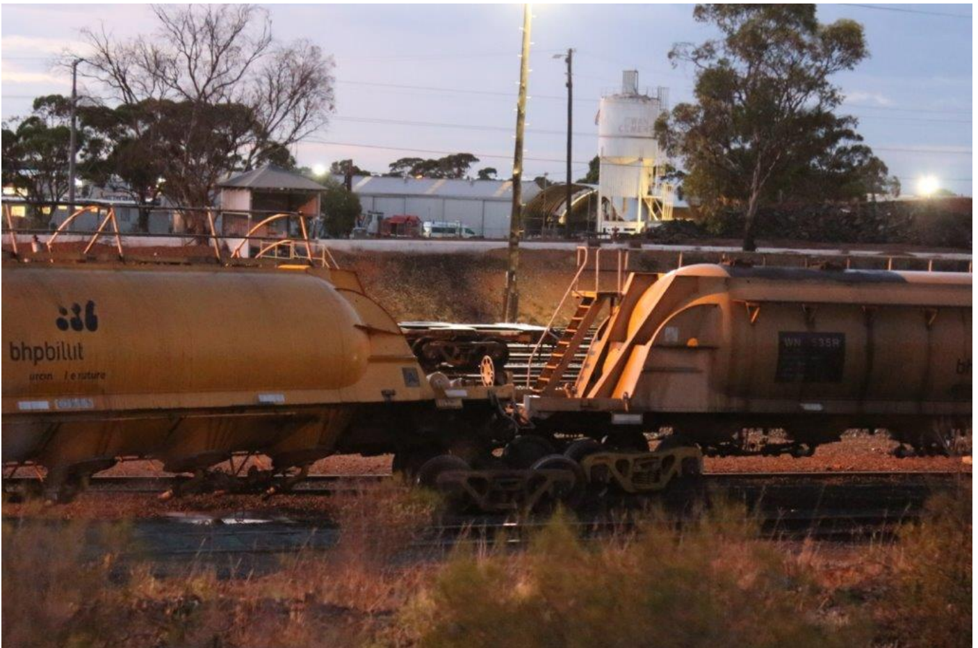
In the early hours of 16 th March, two empty WN nickel wagons on 2479 to Leonora split the points and derailed while departing West Kalgoorlie yard. Rerailing was completed that afternoon. Both photos: Peter Donaghy
