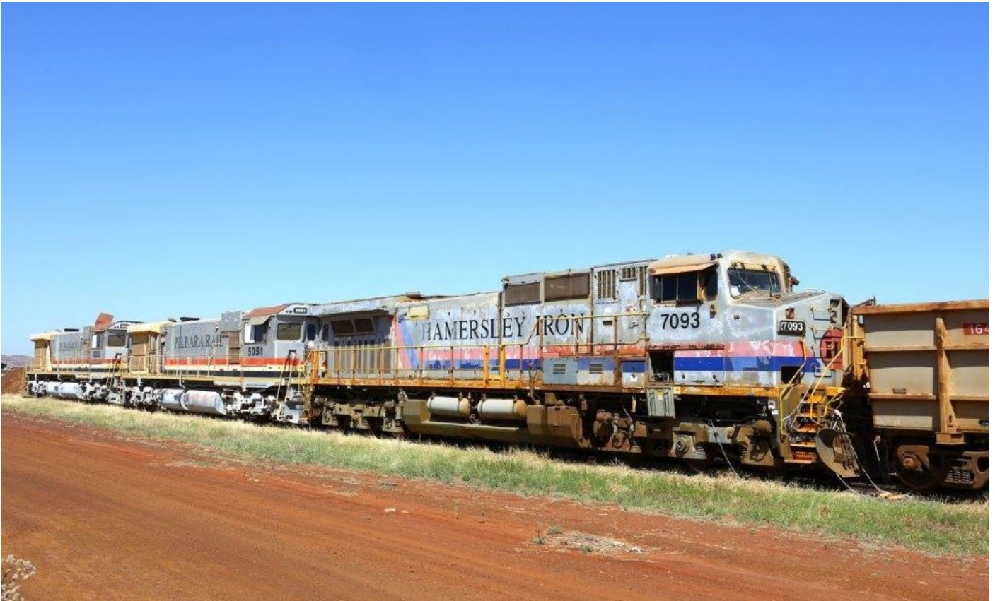
Written-off 7093 (damaged cab from a loader hit) with stored 5051 & 5052, 38 road, 7 Mile, 14 th September. Photo: Pilbara Railways
