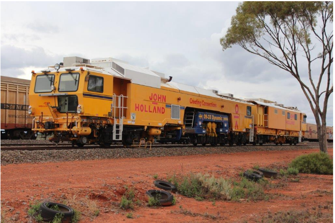
New John Holland tamper on the engineer's siding at Parkeston for commissioning, 11 th November.
