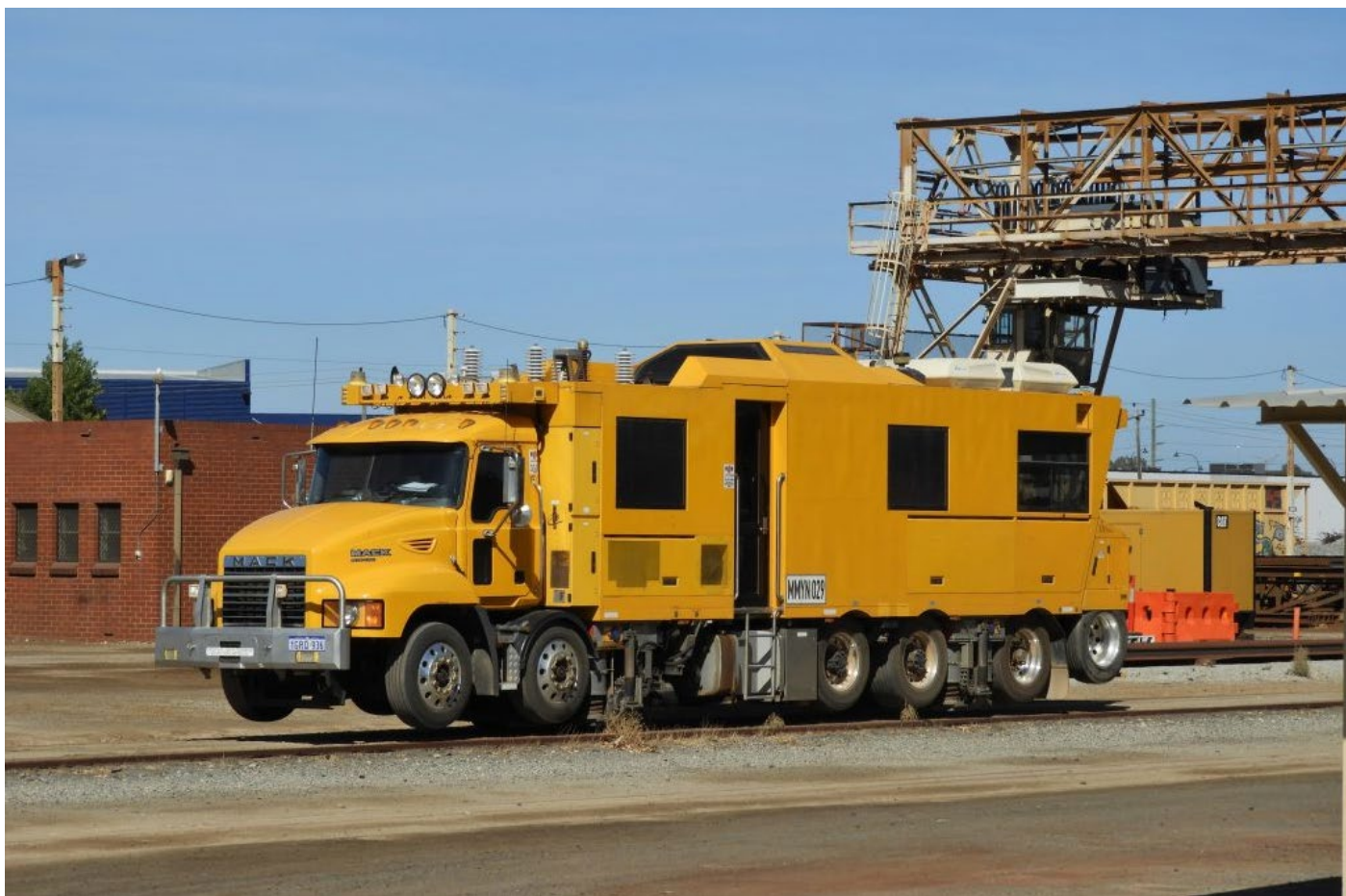
Road-rail MMY029 Sperry rail flaw detection vehicle, Flashbutt yard, Midland, 24 th February.
