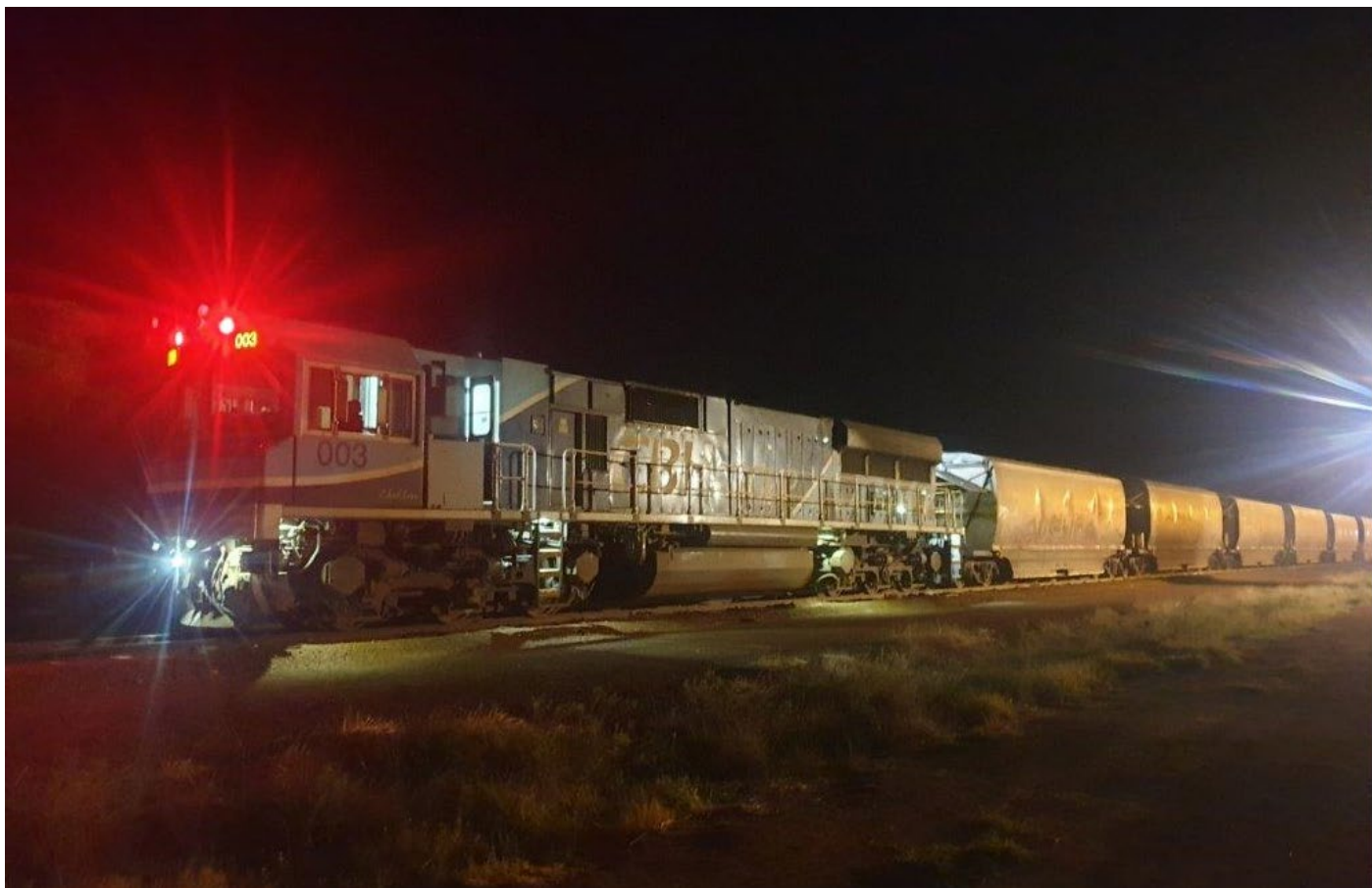
CBH003 stands at Muckinbudin with 6K63, 12 th April. CBH014 will pull the train forward to release CBH003 to the loop; CBH003 will then attach to the front of CBH014 to lead 6K64.
