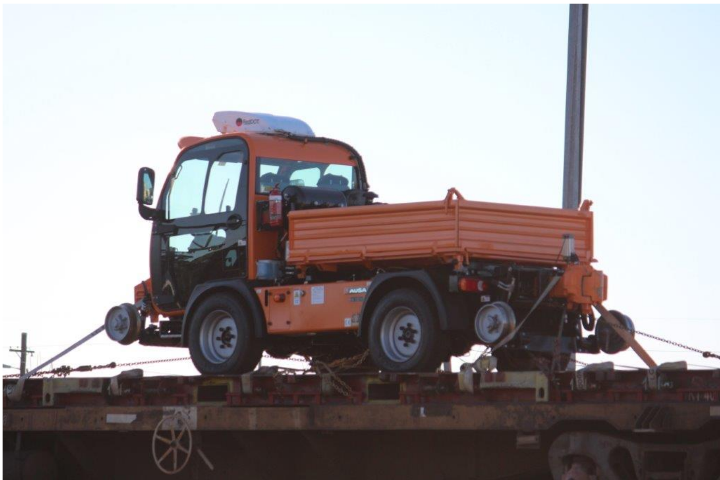
A small road-rail tip truck on 6PS7, West Kalgoorlie, 6 th April. Note the coupler on each end.
