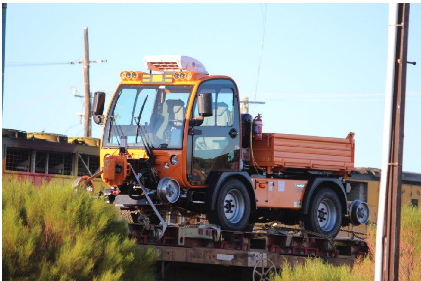
A small road-rail tip truck on 6PS7, West Kalgoorlie, 6 th April. Note the coupler on each end.
