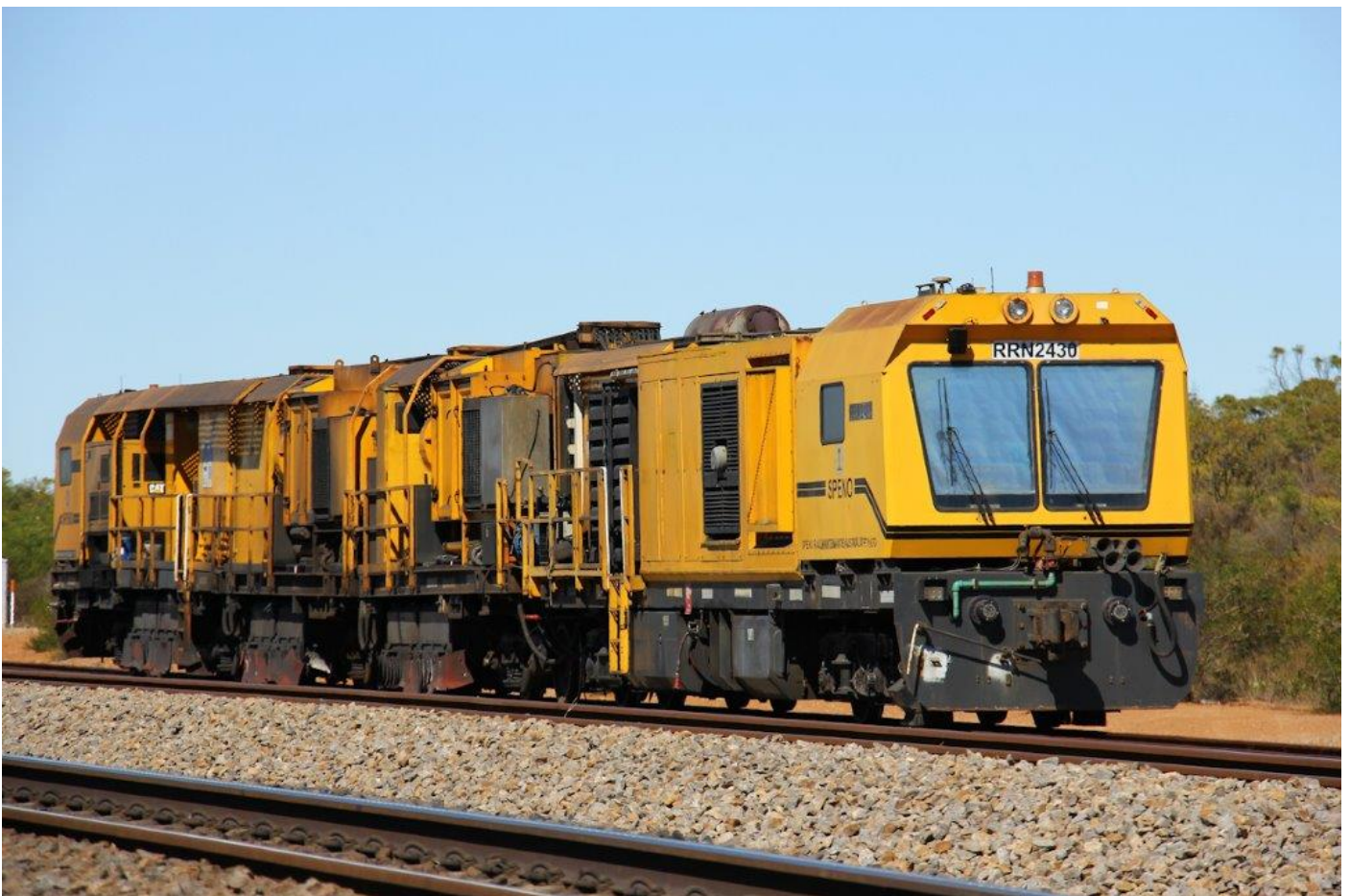
RRN2430 Speno rail grinder at Northern Gully, 26 th April.
