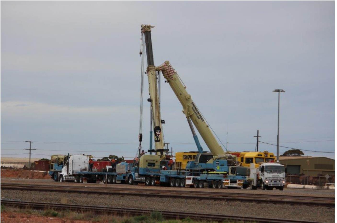
The cranes are being packed away at West Kalgoorlie after lifting Q4011 to allow some temporary bogie/underbody repairs. The Q was returned to Perth that night for workshops attention, 29 th April. Both photos: Peter Donaghy
