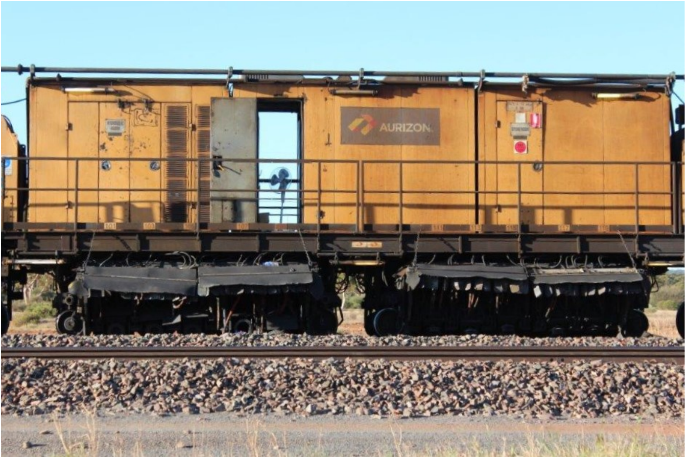
The spark guards on one of the grinding units are raised for maintenance, 2 nd May. Photo: Peter Donaghy
