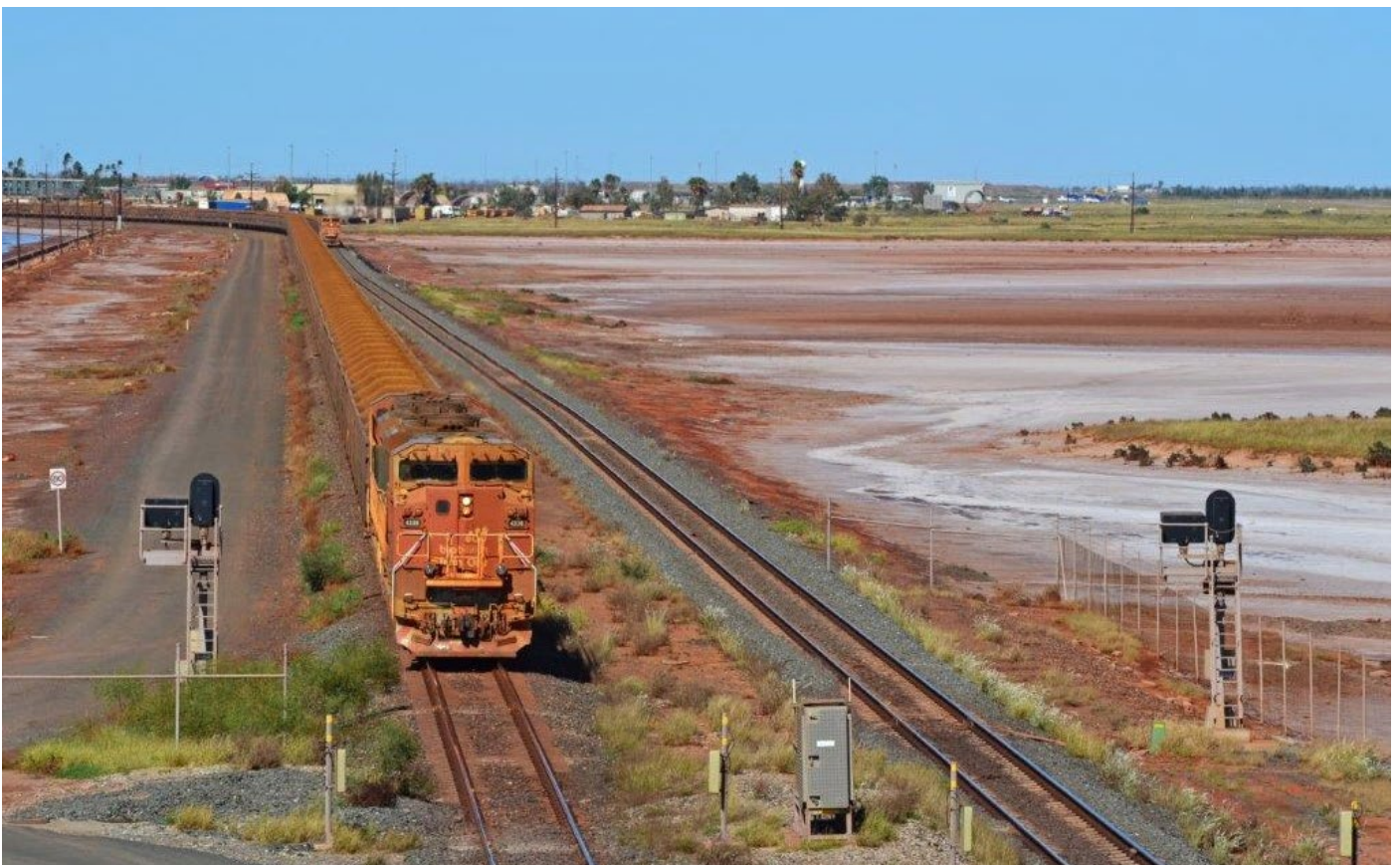
4338 & 4334 on the East Main, 4344 & 4442 on the West Main, two 134-car single rakes split at Mooka Staging facility on the outskirts of town. Both trains take advantage of the bi-directional signalling to approach Hedland Yard together, 29 th May.
