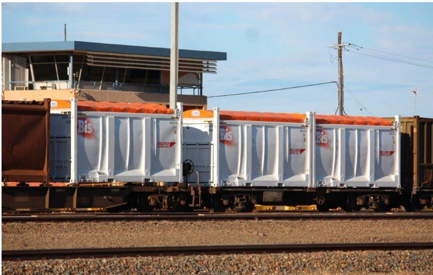
BIS trialled two new sulphur containers earlier this year and has now introduced a couple of dozen into regular use. Three CIMC-built BICN containers are seen in a block on 6029, West Kal, 22 nd June. Photo: Peter Donaghy
