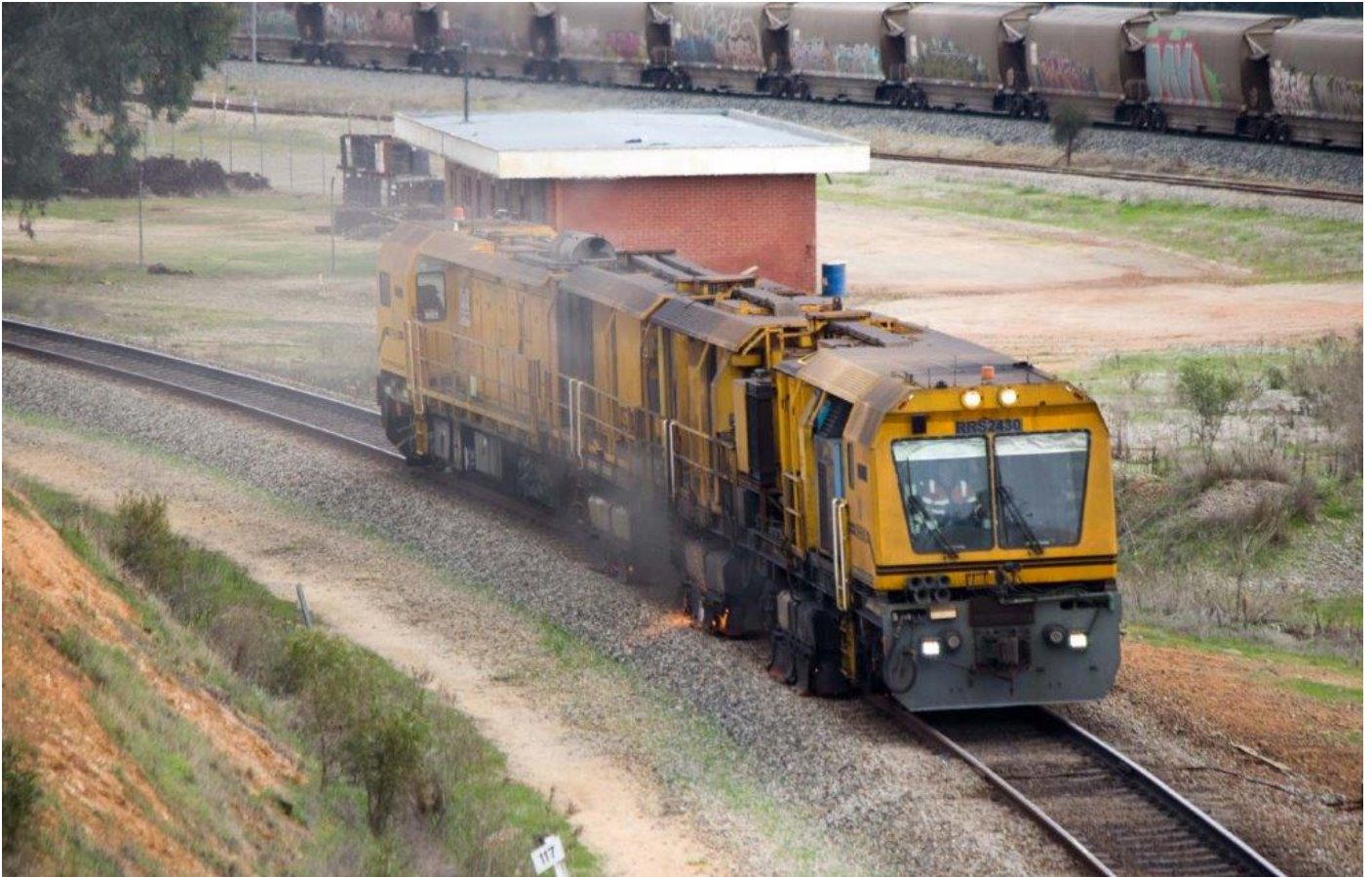
Speno rail grinder RRS2430 at work reprofiling the rail head, Avon Yard, 18 th July.
