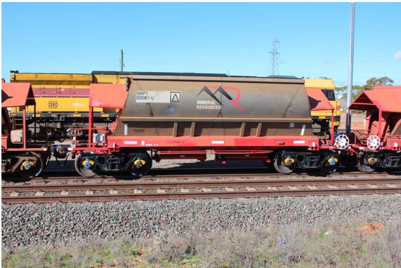
Repaired MHPY81 on 6PM7 at West Kal, 6 th July – damaged in the Salmon Gums derailment eight months earlier.
