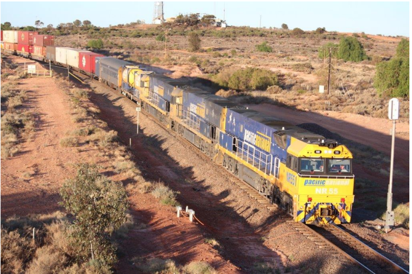
PN are trialling in-line fuelling again – NRs 55, 92 & 94 lead two tanks on 2MP5 approaching Kalgoorlie, 29 th April. Both photos: Peter Donaghy
