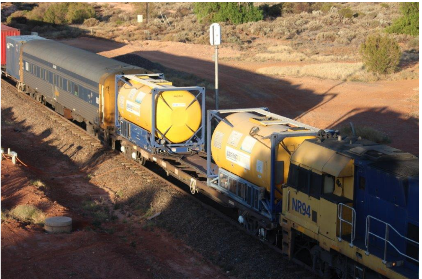
PN are trialling in-line fuelling again – NRs 55, 92 & 94 lead two tanks on 2MP5 approaching Kalgoorlie, 29 th April. Both photos: Peter Donaghy
