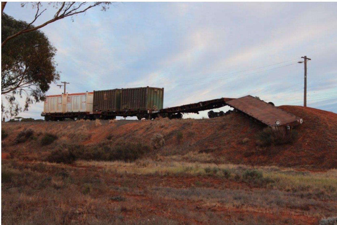
AQRY1001 has over-run the end of the shunt neck, West Kalgoorlie, 10 th May.
