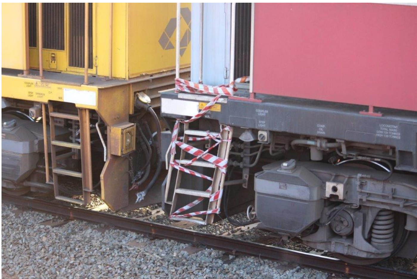
MRL006's steps, damaged several months ago in a level crossing incident. The mid-loco steps have since been replaced with a set probably taken from a sister unit. Both photos: Peter Donaghy
