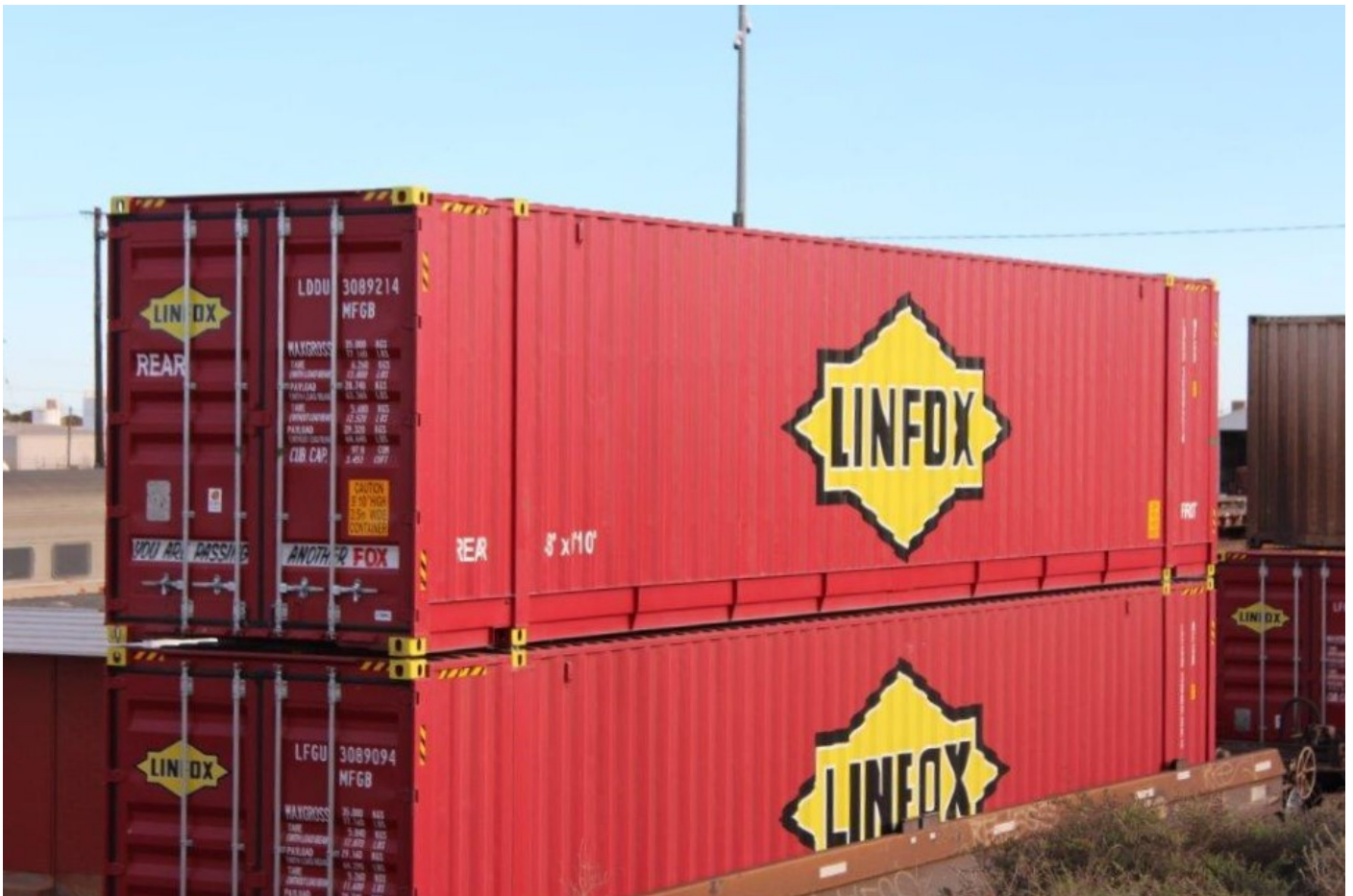
Among 280 new containers purchased by Linfox late last year are eight LDDU-coded boxes with doors at both ends. LDDU3089214 on 7SP5, West Kal, 11/5. Note "Front" and Rear" marked on box. Both photos: Peter Donaghy
