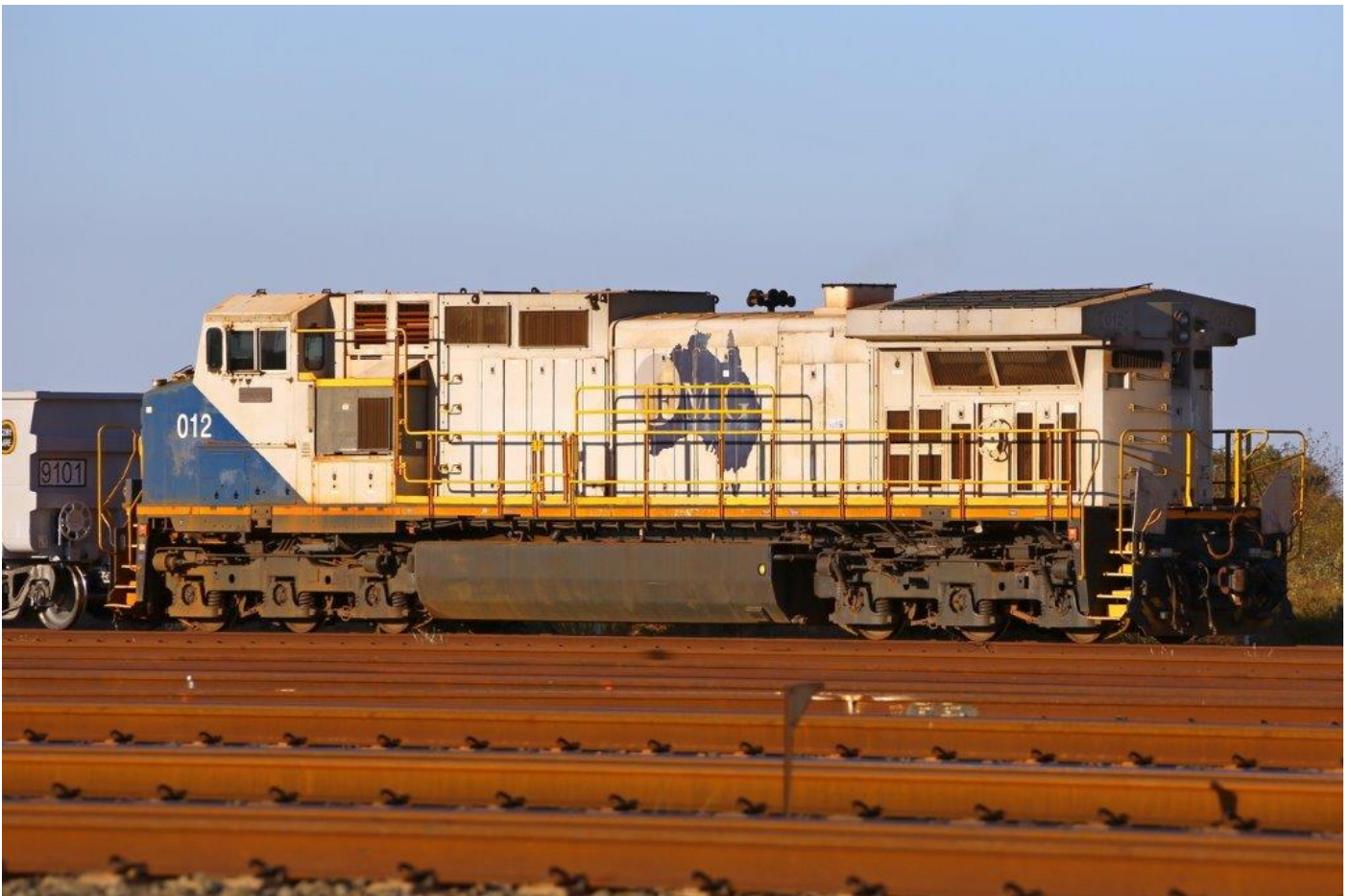
C44-9W 012 "Peter Tapine" sports modified handrails, kick rail and steps, 5 th May. Both photos: Pilbara Railways
