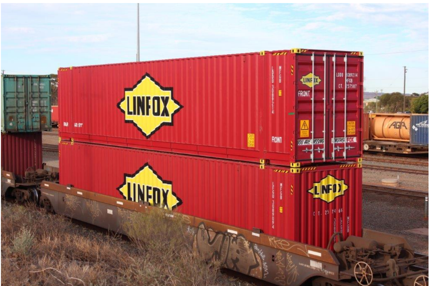
Among 280 new containers purchased by Linfox late last year are eight LDDU-coded boxes with doors at both ends. LDDU3089214 on 7SP5, West Kal, 11/5. Note "Front" and Rear" marked on box. Both photos: Peter Donaghy
