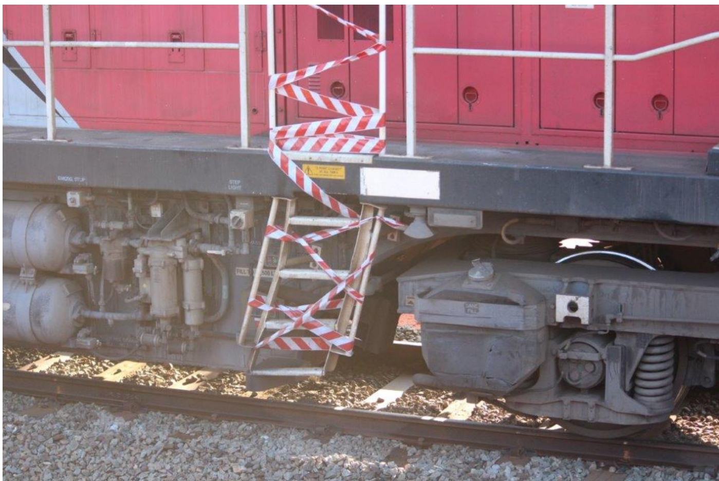
MRL006's steps, damaged several months ago in a level crossing incident. The mid-loco steps have since been replaced with a set probably taken from a sister unit. Both photos: Peter Donaghy
