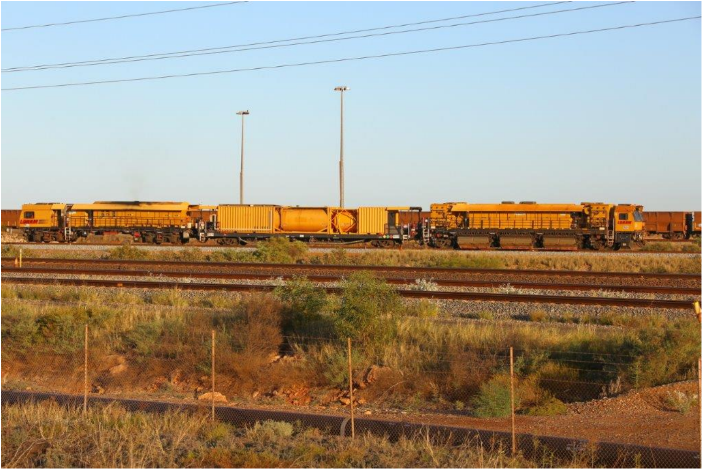
Overview of the Loram RG24 rail grinder (above) and the grinding and driving module (below), Nelson Point yard, 22 nd June. Both photos: Pilbara Railways
