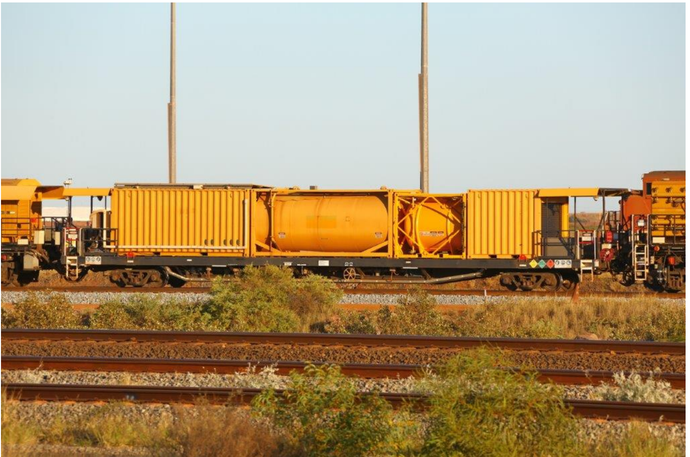
Loram RG24 power generating and driving module (above) and workshop, water and fuel tank wagon (below), at Nelson Point yard, 22 nd June. Both photos: Pilbara Railways
