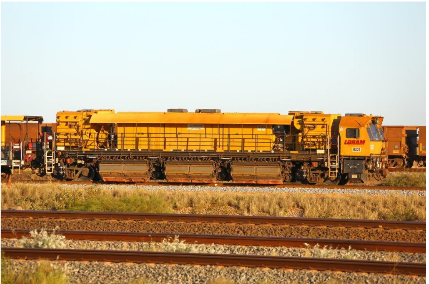
Overview of the Loram RG24 rail grinder (above) and the grinding and driving module (below), Nelson Point yard, 22 nd June. Both photos: Pilbara Railways
