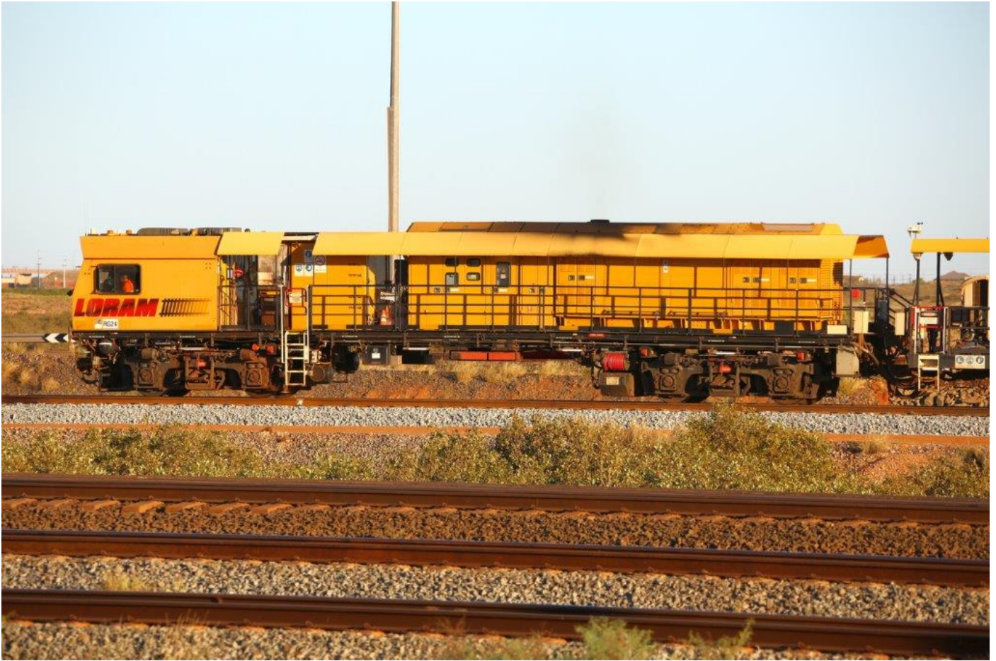
Loram RG24 power generating and driving module (above) and workshop, water and fuel tank wagon (below), at Nelson Point yard, 22 nd June. Both photos: Pilbara Railways
