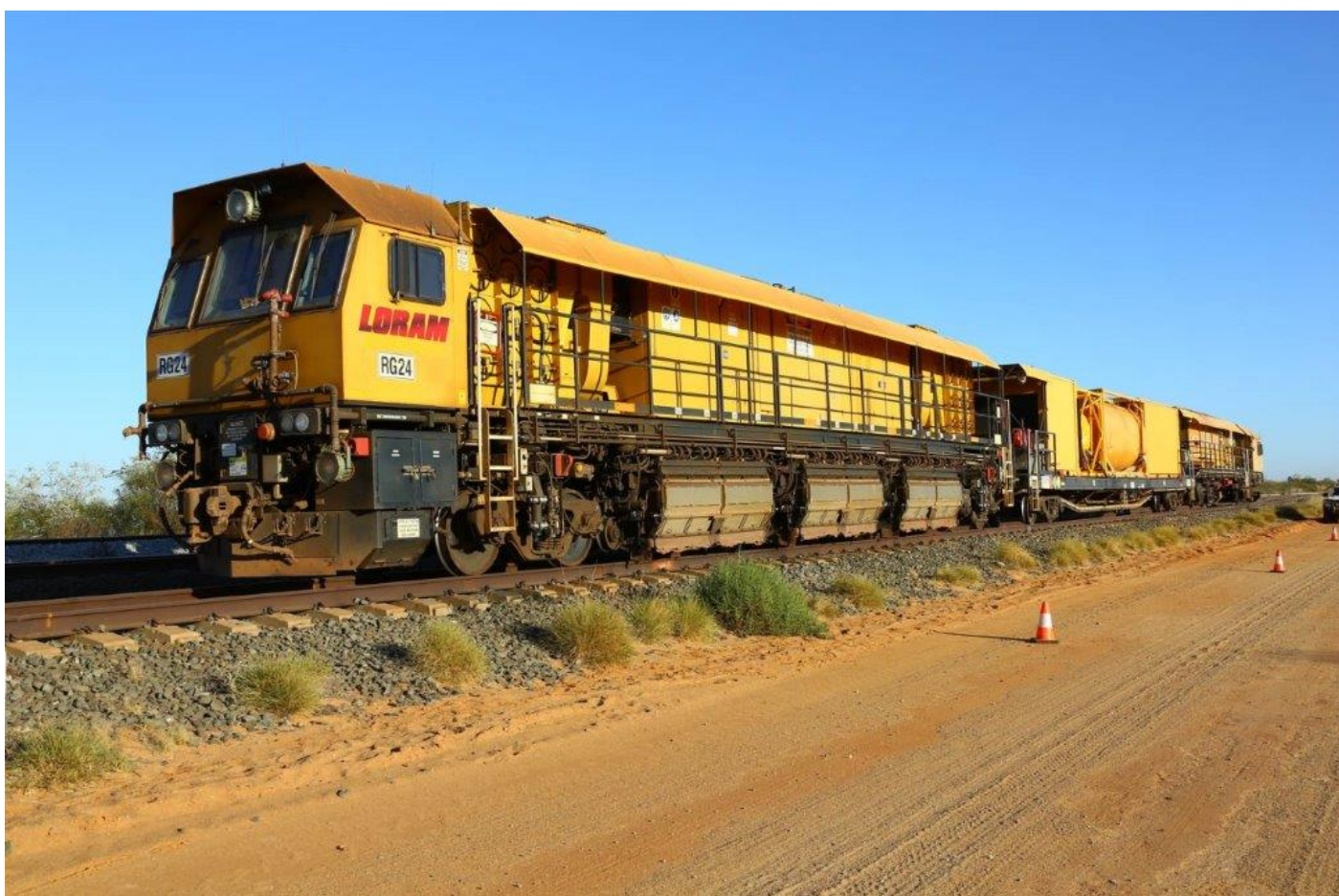
Loram RG24 (ex Aurizon MMY521), an RGS type 24 stone grinder, at Tabba, 12/9.
