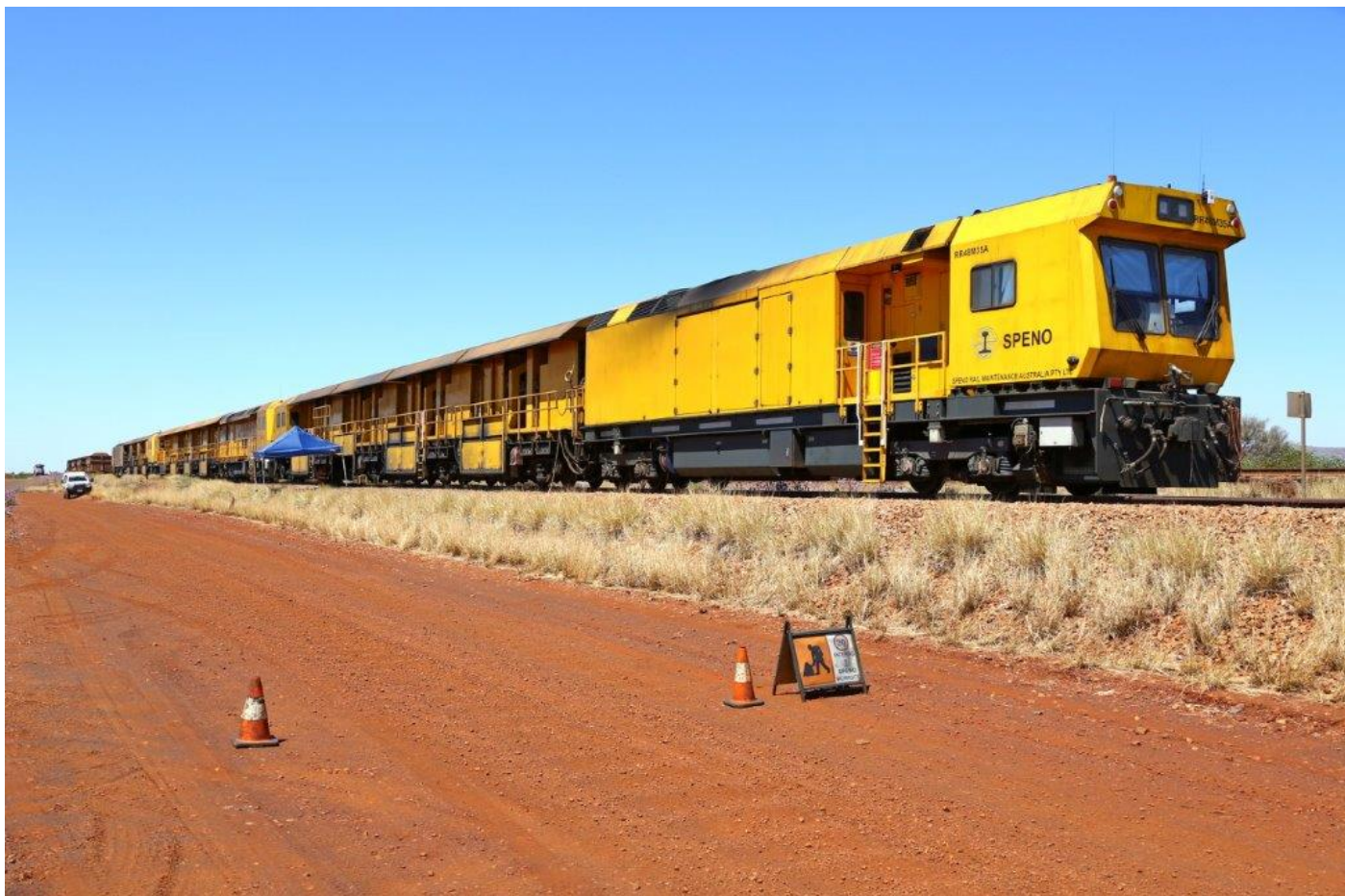
All three Speno grinders undergoing maintenance, Gidji siding, 12/9; RG3 (48 stone), RG5 & RG4 (both 36 stone).
