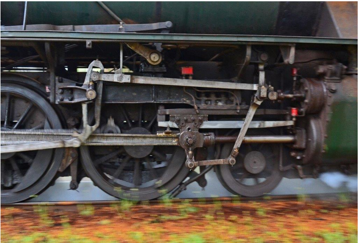
The motion gear on W945 (above), as it hauls a Steam Ranger passenger service with former Midland Railways F40, 1 st November. Both photos: Mark Bennett
