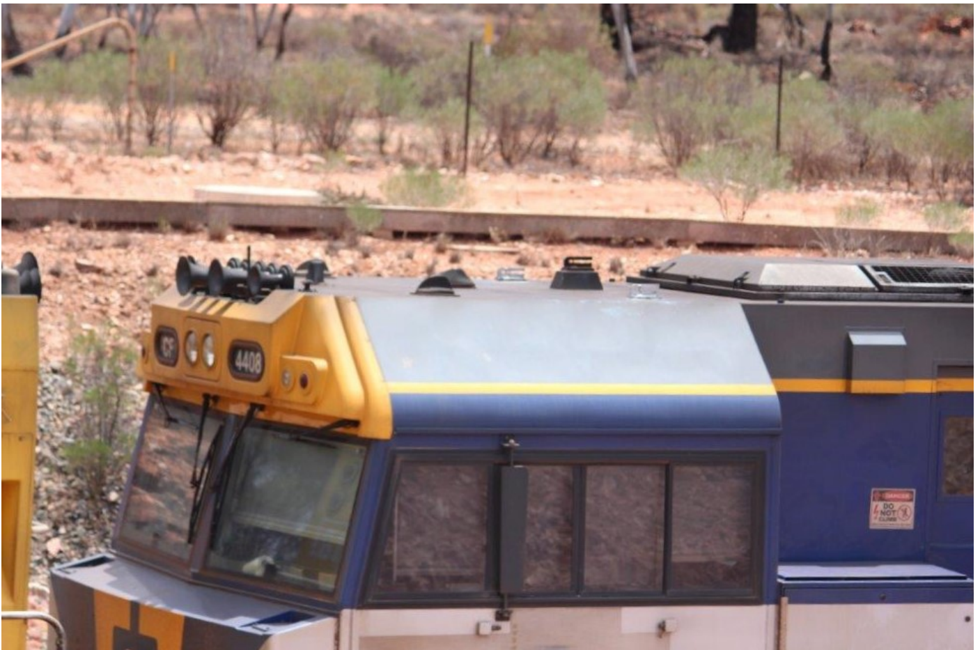
The two new small antennae on the roof of CF4408 are part of the newly-installed distributed power unit, 15/11.
