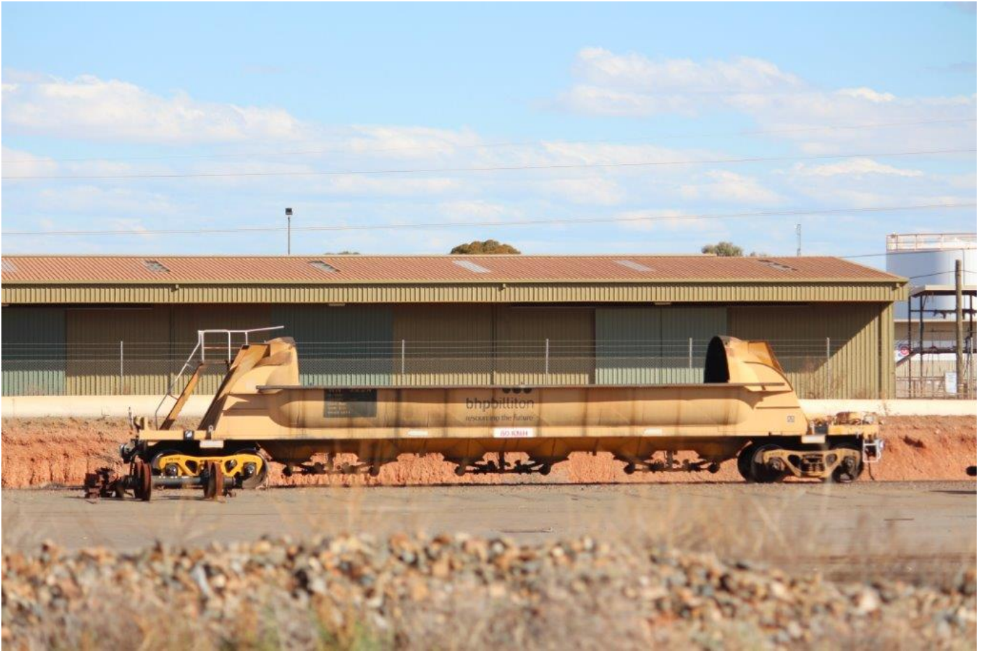
WN529 buckled upper portion during unload, awaits construction of a new top, West Kalgoorlie, 13 th November.
