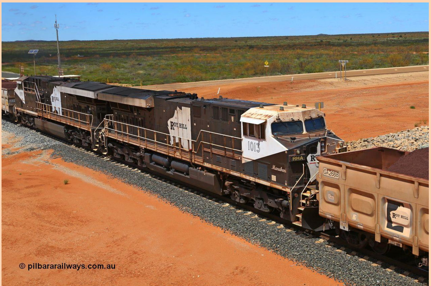
A Roy Hill loaded at the highway bridge which is their 18 km post and a pair of GE ES44ACi units RHA 1006 and RHA 1004 lead their train with mid-train remotes RHA 1013 'Marubeni' and RHA 1019.
