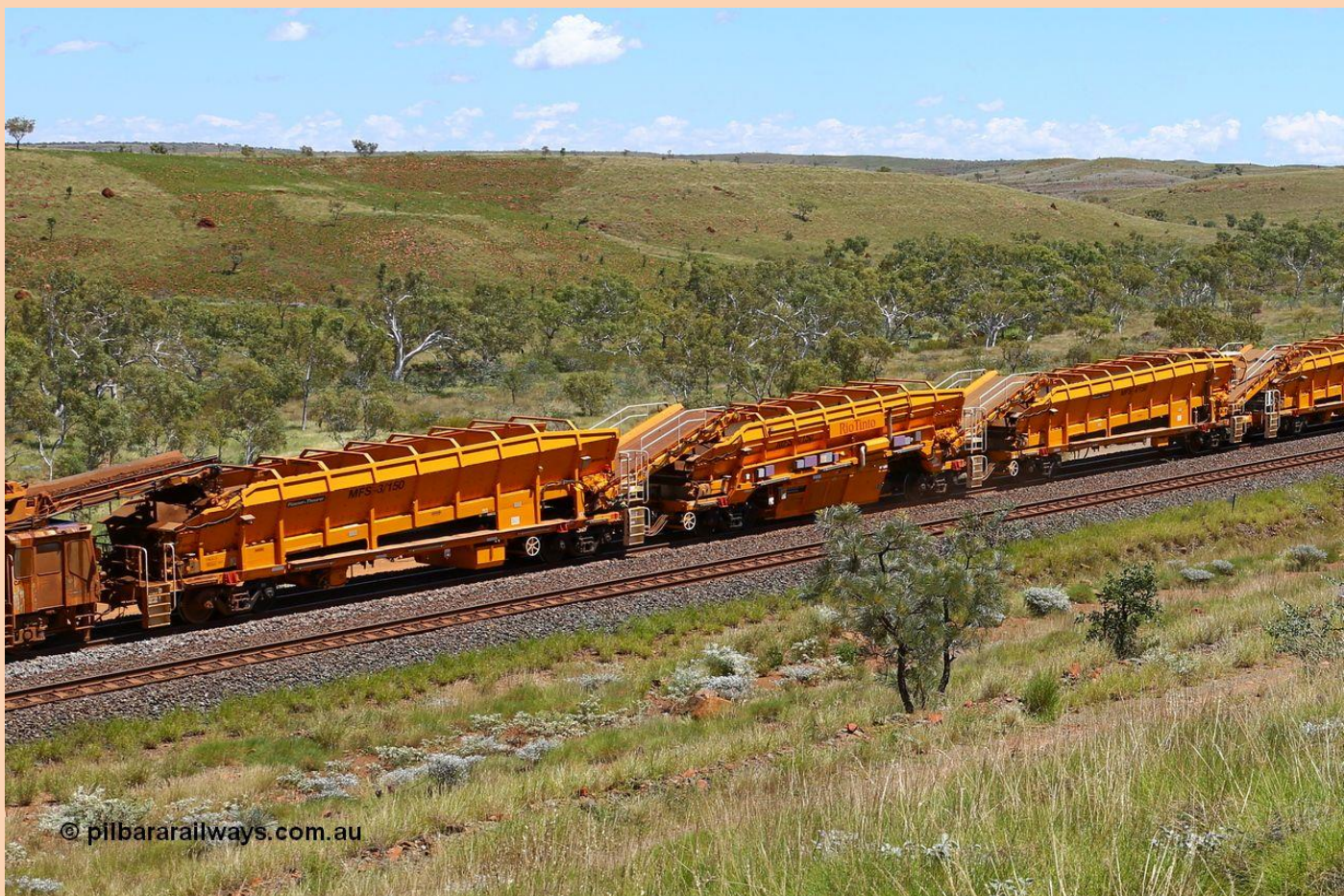
At Green Pool and a trailing shot of another stabled AutoHaul™ train with GE ES44DCi 8165 leading two GE C44-9W units 7059 in Pilbara Iron livery and 7080 in original Hamersley Iron. Below are one of four sets of Plasser & Theurer built MFS 3/150 material conveyor and hopper units on Rio Tinto's ballast cleaning train.
