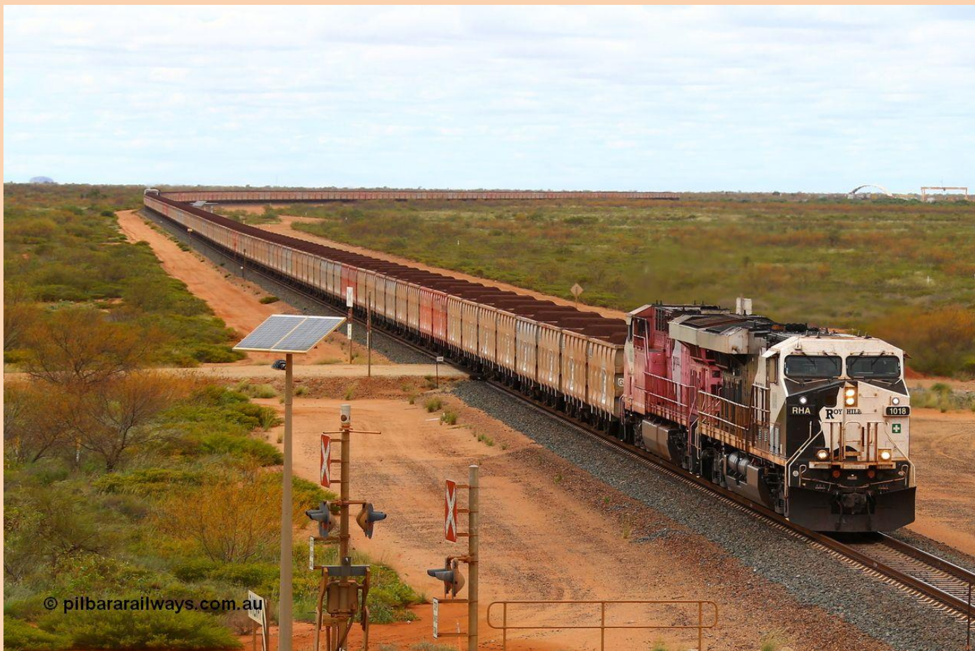
Roy Hill loaded arrives at their Great Northern Highway road overpass with GE ES44ACi units RHA 1018 and RHA 1022 on the point and RHA 1016 and RHA 1017 as the mid-train remote units. BHP and Roy Hill both use mid-train or DPU power.
