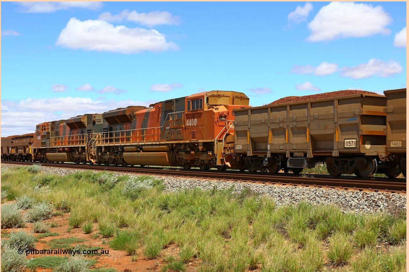
Above mid-train units on the loaded with a broken rail detection waggon (or BRD) 11571 with 4400 and 4405 'Dusty'. And below is another BRD waggon 11679. BHP intend on doing some 70 waggons with this Siemens technology. 11679 is a 2020 build from QRRRC Qiqihar Rolling Stock Co. of China.
