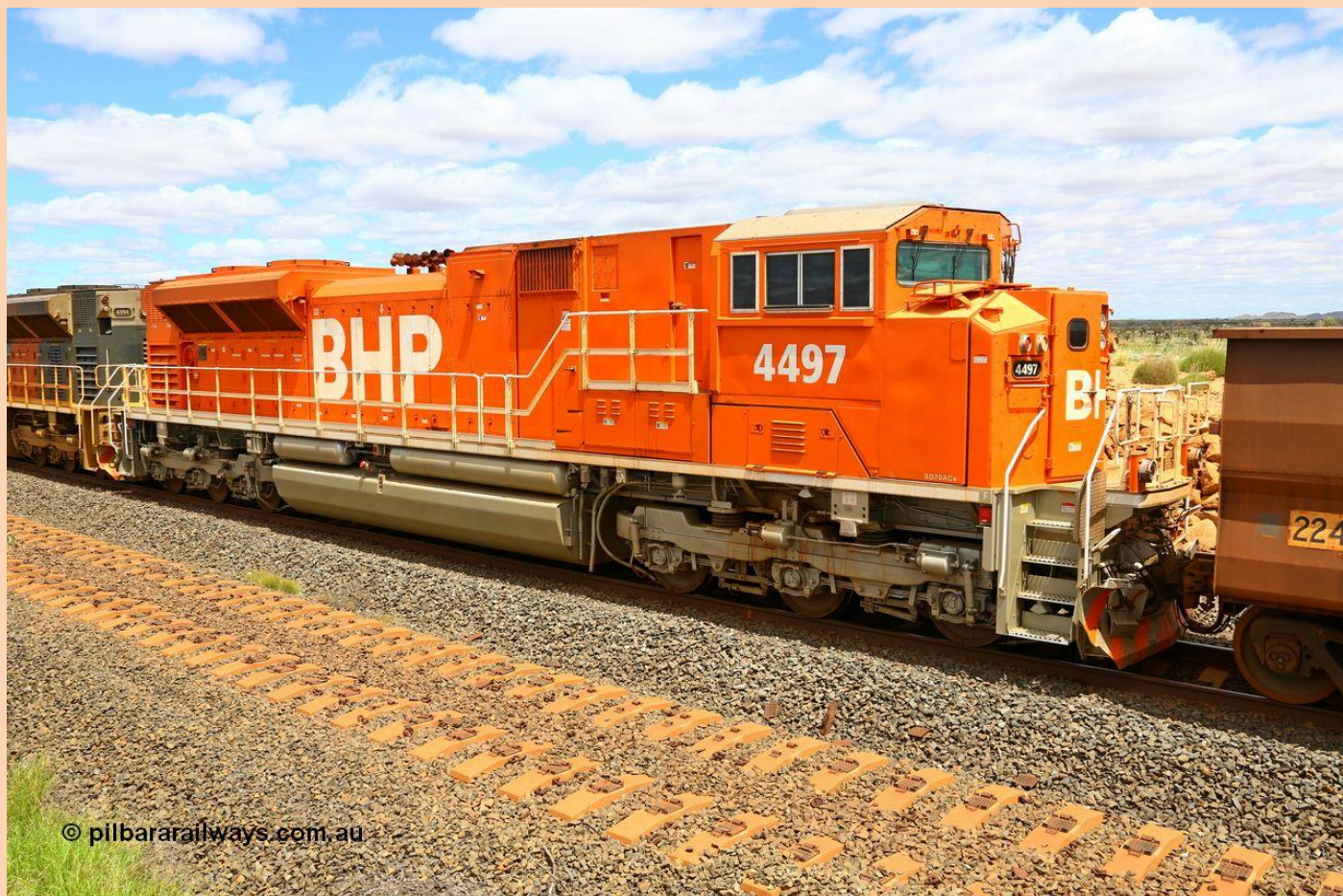
An empty train wait line clear behind EMD SD70ACe/LCi unit 4394 and new liveried unit 4497 with the original formation in the foreground which became redundant with the duplication. 4497 is the highest numbered locomotive from the latest delivery for BHP and carries serial number 20198860-006 build in May 2020 by Progress Rail, Muncie USA.
