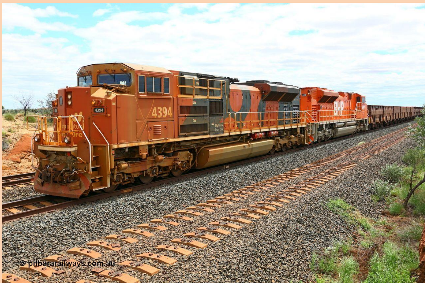
An empty train wait line clear behind EMD SD70ACe/LCi unit 4394 and new liveried unit 4497 with the original formation in the foreground which became redundant with the duplication. 4497 is the highest numbered locomotive from the latest delivery for BHP and carries serial number 20198860-006 build in May 2020 by Progress Rail, Muncie USA.
