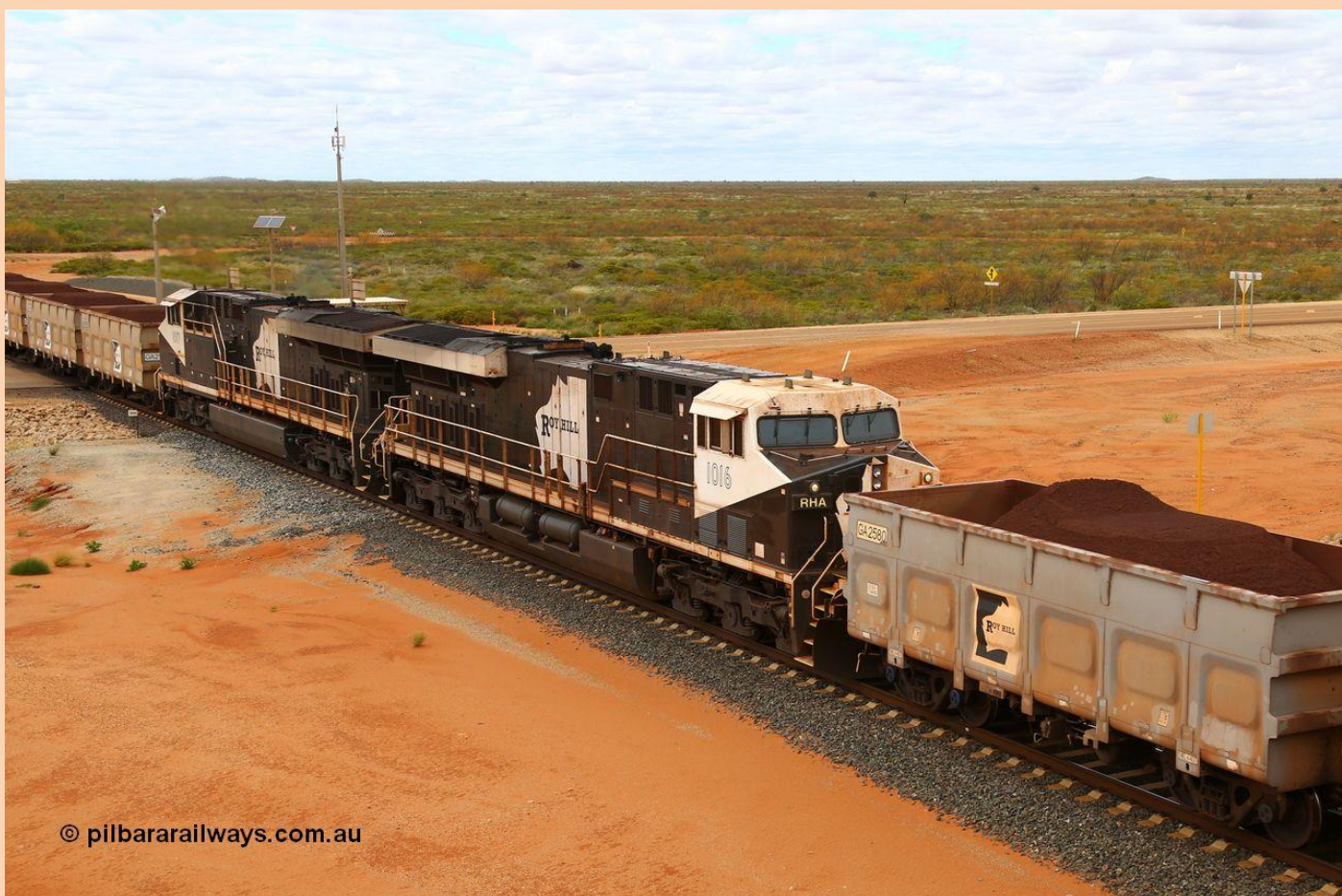
Roy Hill loaded arrives at their Great Northern Highway road overpass with GE ES44ACi units RHA 1018 and RHA 1022 on the point and RHA 1016 and RHA 1017 as the mid-train remote units. BHP and Roy Hill both use mid-train or DPU power.
