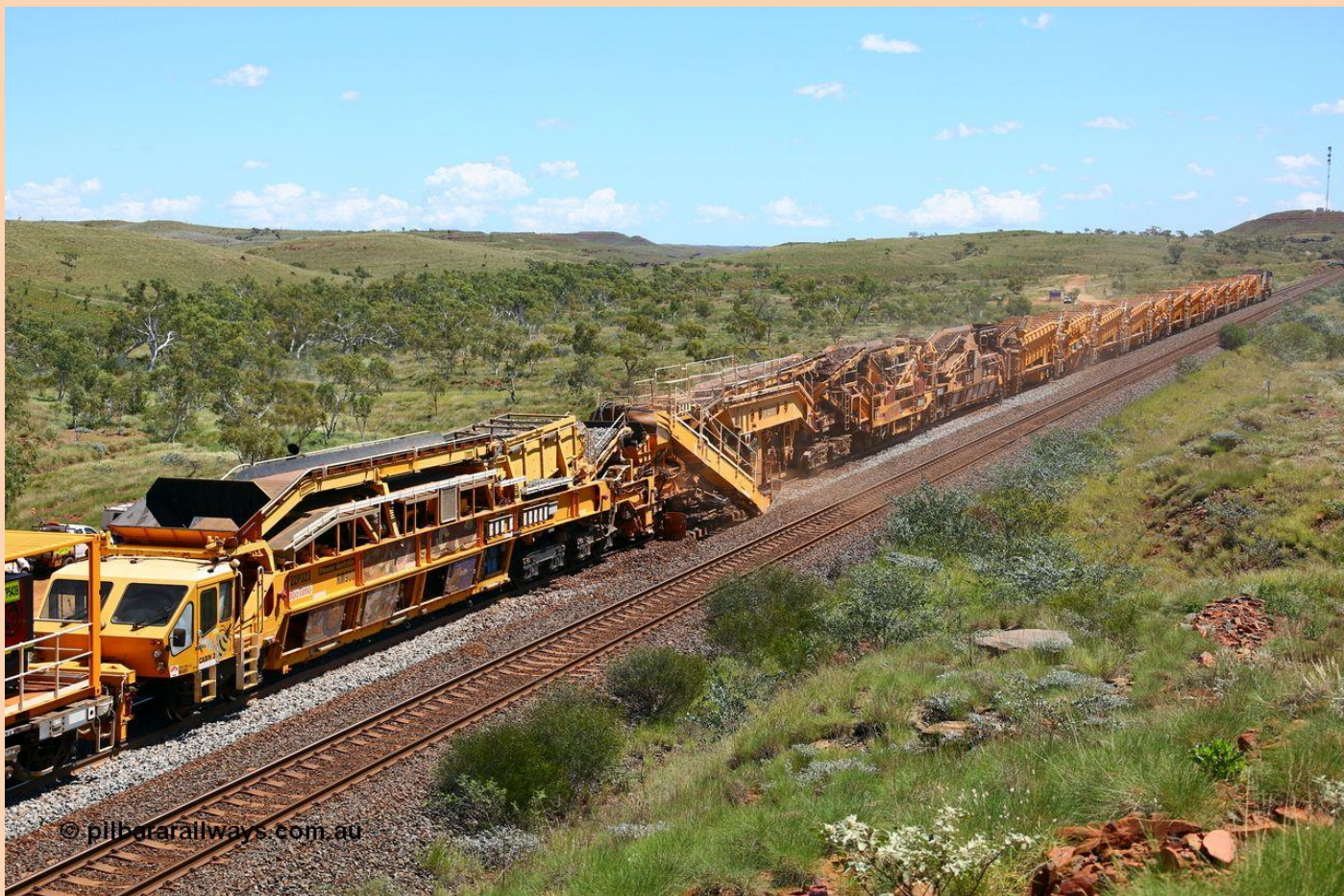
Rio Tinto's Plasser Australia built RM900 ballast cleaning machine with serial M491 with the four sets of the MFS 3/150 units cleaning ballast near the 94 km. Below is Pilbara Iron liveried GE C44-9W unit 7056 on the rear of the ballast cleaning train as it works north near the 94 km.
