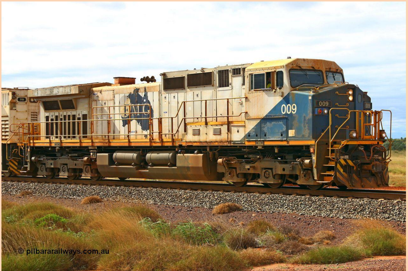
FMG GE C44-9W unit 009 serial 58186 leading an empty train at Indee Rd shows the handrail modifications the fleet has gained. Below on the 21 st March 2021 a Roy Hill empty approaches the highway bridge behind GE ES44ACi units RHA 1008 and RHA 1009 'Posco'.
