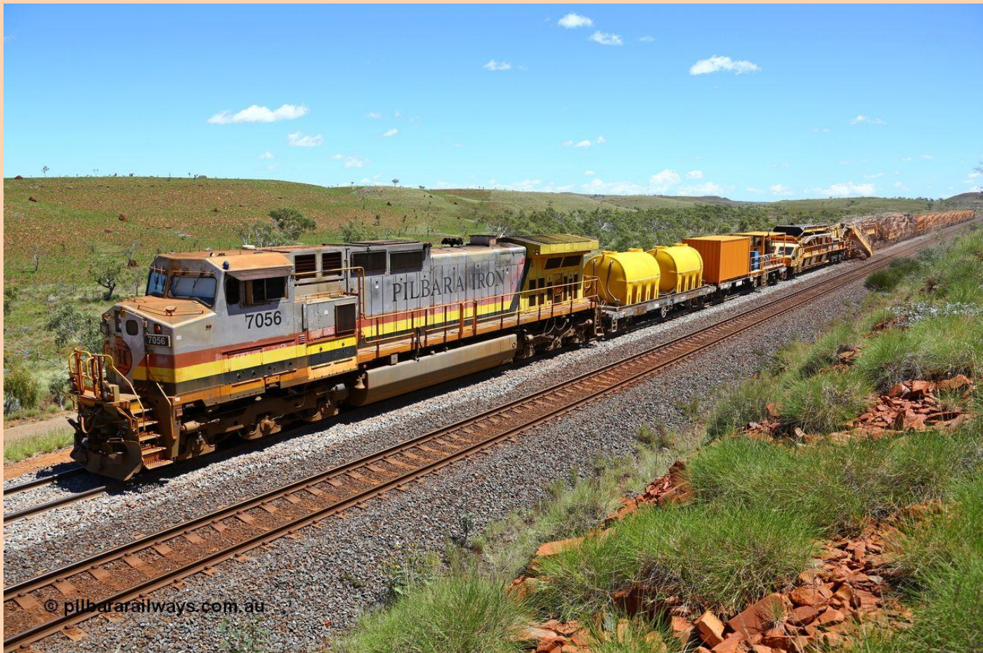
Rio Tinto's Plasser Australia built RM900 ballast cleaning machine with serial M491 with the four sets of the MFS 3/150 units cleaning ballast near the 94 km. Below is Pilbara Iron liveried GE C44-9W unit 7056 on the rear of the ballast cleaning train as it works north near the 94 km.
