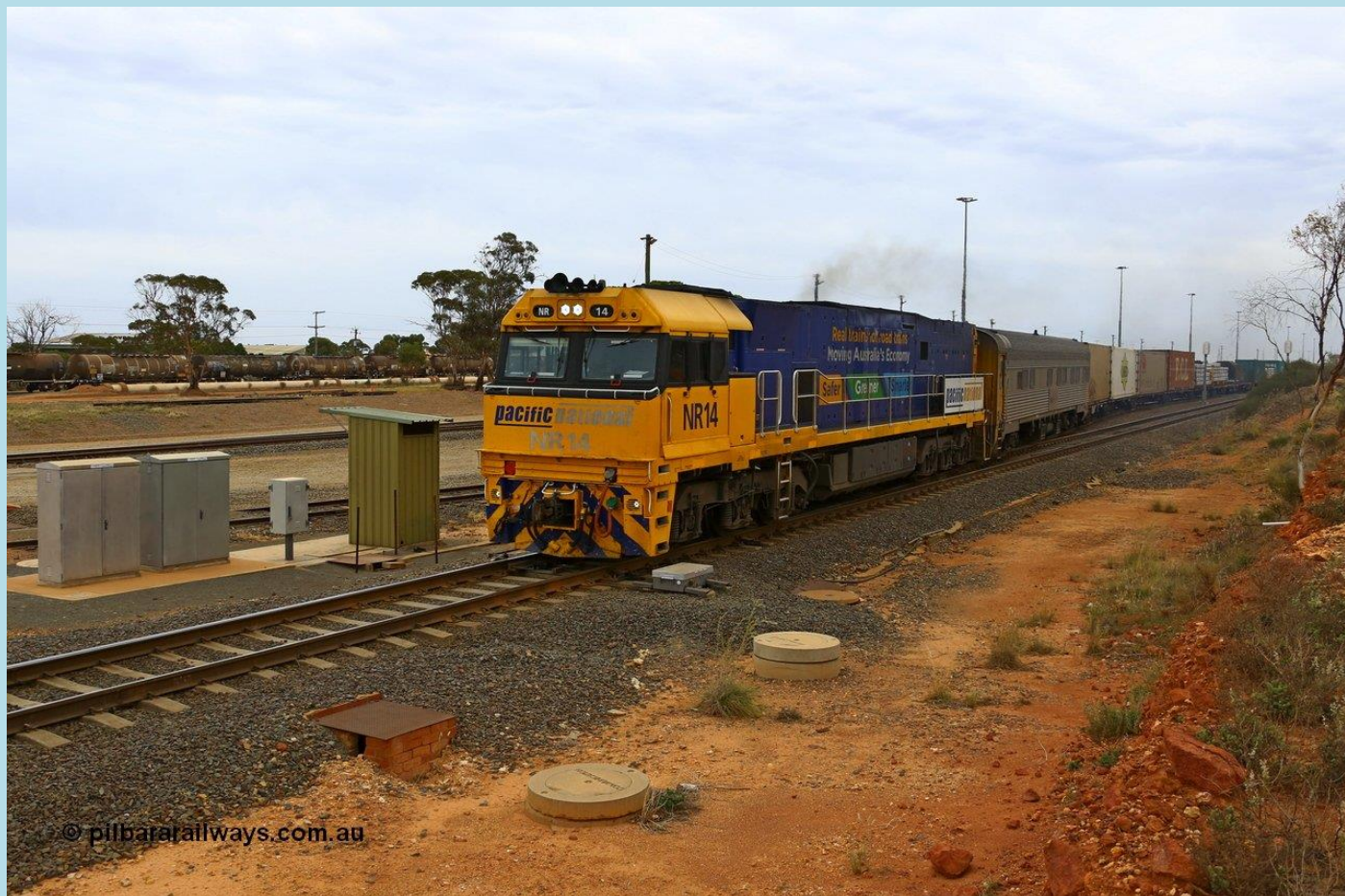
West Kalgoorlie, PN priority service 4MP7 behind NR 26 and NR 63 with 38 vehicles for 3244 t and 1760 m in length. Below 4PM4 with solo NR 14 and RZAY 985 with 46 vehicles for 1670 t and 1043 m.
