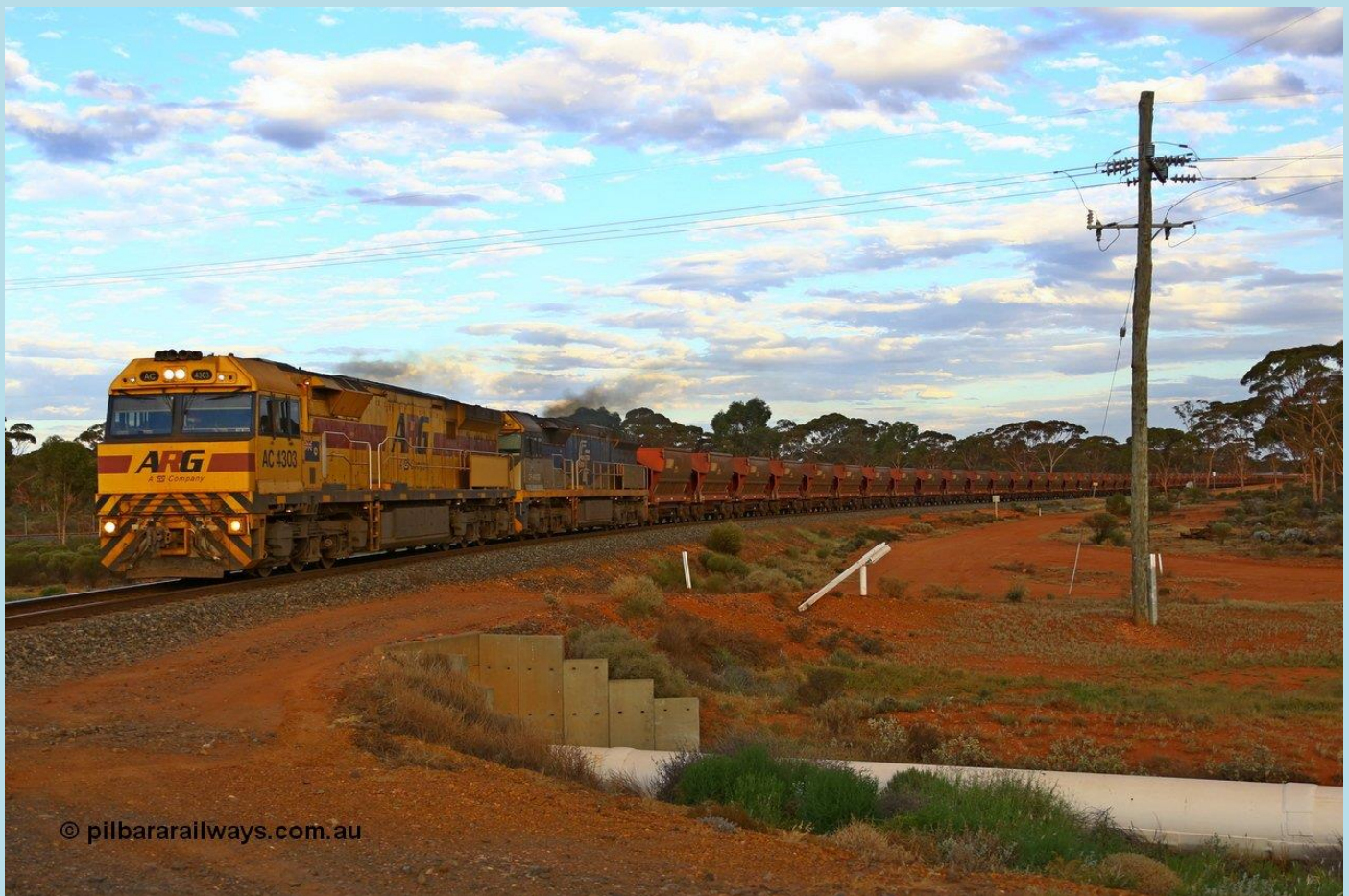
At Binduli 4032 empty ore train powers around the west leg behind AC 4303 and CF 4406 'Kiwi' with mid-train units AC class leader AC 4301 and CF 4408 'Mentor'. CF 4406 has been in the Pilbara previously. The AC's are AC43aci, the CF's are AC44aci.
