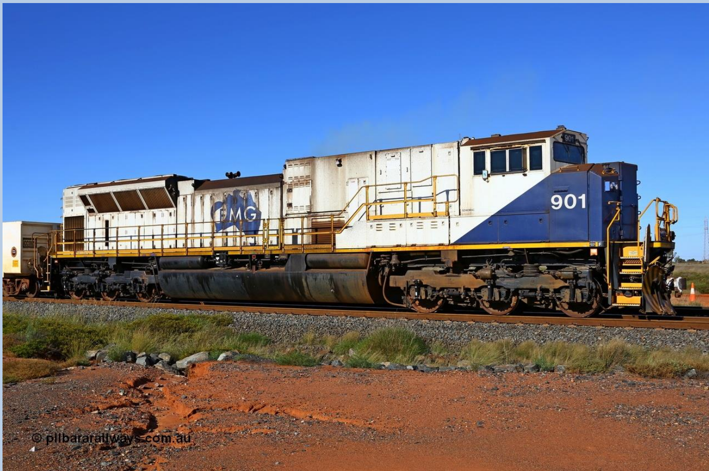
Kanyirri Yard and FMG loaded train behind C44-9W 011 and SD9043MAC 905 power through to the port. Below port pilot loco SD90MAC-H2 901 (re-motored with 710) stands with compressor sets at the port.
