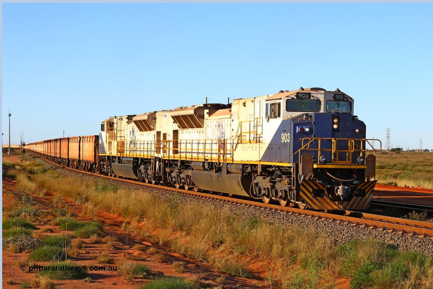
Empty departure from FMG port with two SD90MAC-H2 units (both re-motored with 710s) 903 and 902. Below a pair of light engines C44-9W 011 and SD9043MAC 905 head to Kanyirri for trip servicing.
